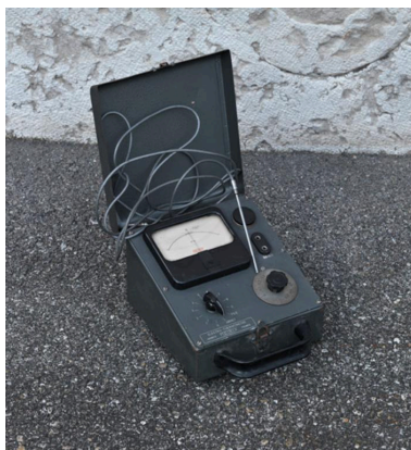
Turbidimeter "Hach" Phot. Eric Dessert IVR82_20126901342NUCA
