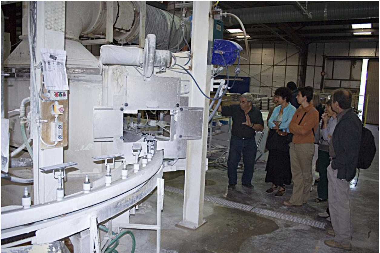
Emallage : machine carrousel
